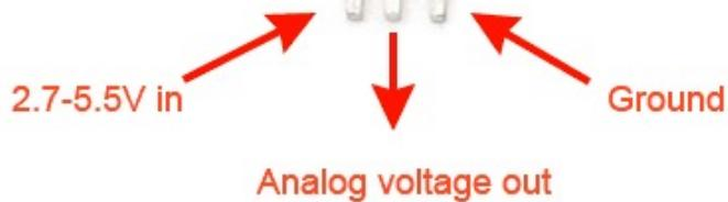
A Temperature sensor like TM36 use a solid-state technique to determine the temperature.
